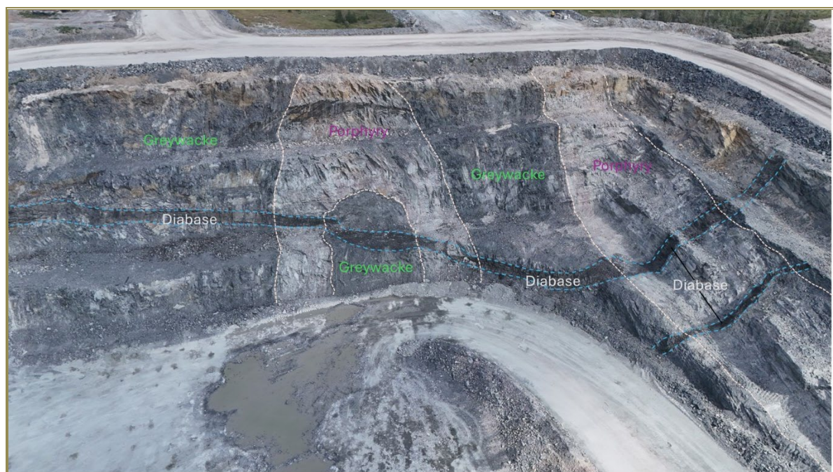
Figure 7-13: Greenstone Mine, East Pit at Southeast Corner—Folded Porphyry and Greywacke Units Crosscut by Younger Diabase Dikes
