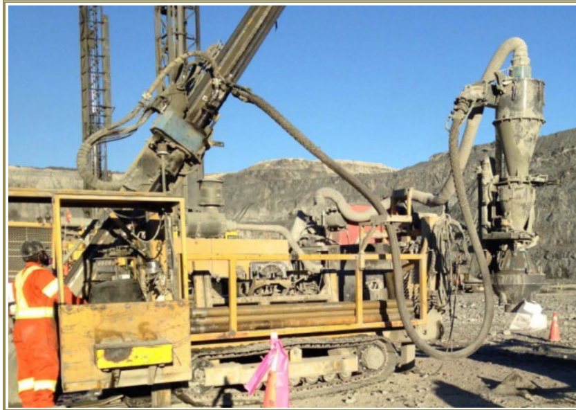
Figure 10-5: Hardab 7000 Maxidrill RC Drill Rig
